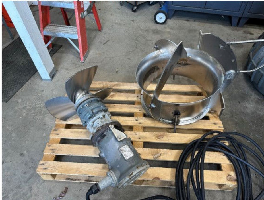
Photo 1. Recycle Wall Pump with broken bracket
