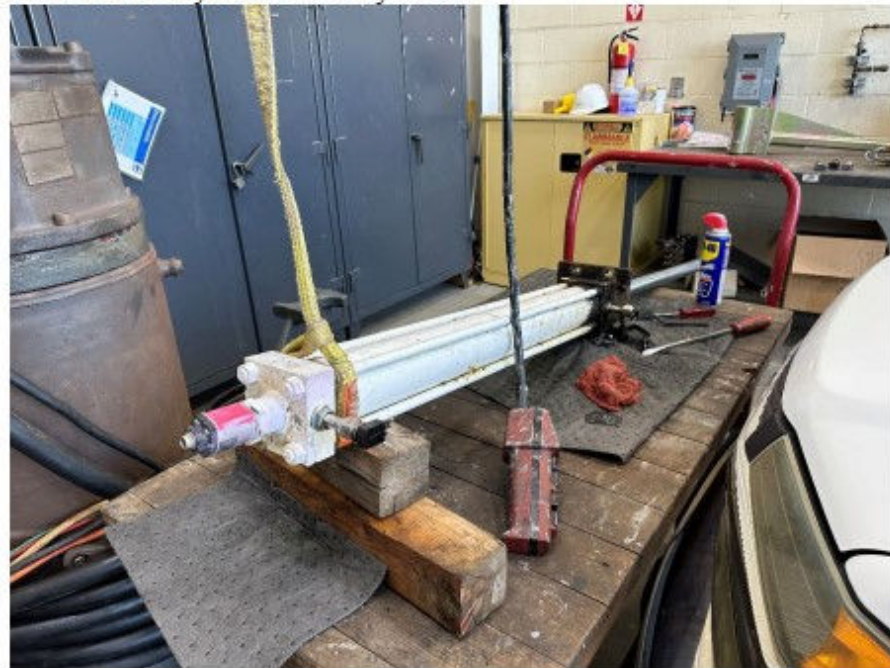
Photo 3. TSB Hydraulic Gate Cylinder.
